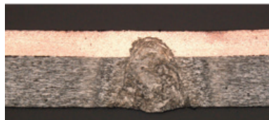
300µm Steel on 2 x 80 µm Cu Lead
