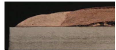
20 x 8µm Cu Foil on 500 µm SS Lead
